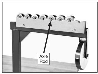
**Figure 10.** Lower wheel assemblies on wheel storage racks.
